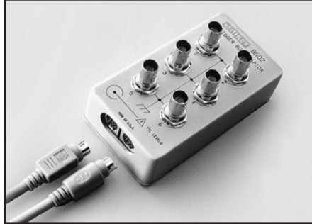
Model 8502: Trigger Link adapter box has two female 8-pin micro DIN connectors to 6 female BNC connectors. Includes an 8501-1 cable. For use with: Series 2000, Series 2400, 7001, 7002
