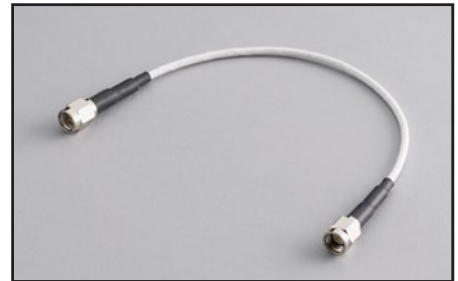
CA-452A: 20.4cm (8 in) RG188 coax cable terminated with an SMA male plug on each end, 50Ω impedance.
