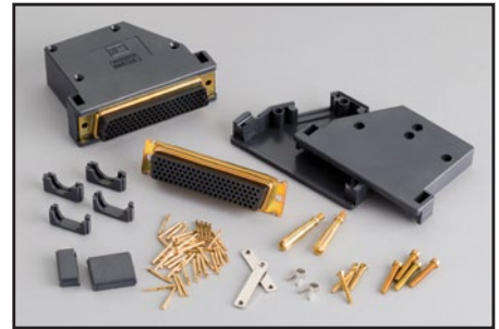
Model 3792-KIT104-R/F: 104-pin female D-sub connector kit that contains two female D-sub connectors with housings and 208 solder-cup contacts. Use for assembly of custom cables, harnesses, and DUT interface compatible with Series 3700A plug-in cards.
