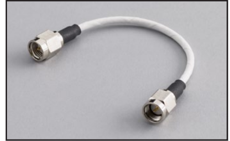
CA-451A: 10.8cm (4.25 in) RG188 coax cable terminated with an SMA male plug on each end, 50Ω impedance.
