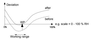
The advantage of the 1-point adjustment is the good measuring result in the working range. But the further away the measurement is from the working point, the greater the deviation can become. The 1-point adjustment should therefore only be used for a relatively narrow measuring range (working range), e.g. clean room applications, air conditioning applications for storage and similar.
