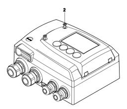
2 Close the service flap and tighten screws (2).
