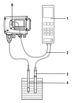
1 Connect Testo handheld instrument 400/650 (1) with connected humidity reference probe (3) (order no. reference set 0699 3656/20) to the service interface (5) of the testo 6681 via the adjustment adapter (2) (connected to the probe socket 1 of the handheld instrument).
