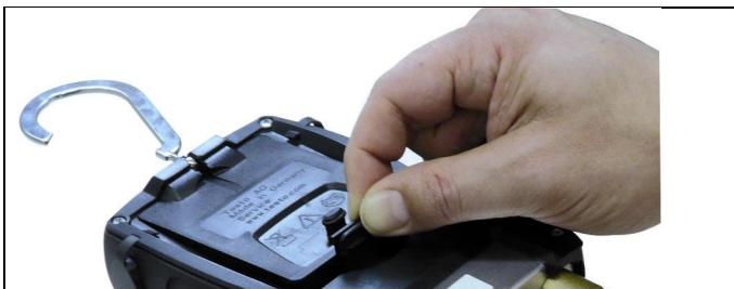
1. Fold out the suspension device, loosen the clip and remove the cover of the battery compartment.
