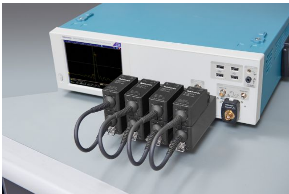
Figure 3: DPO7OE Series supports multiple optical inputs and multi-carrier configurations
