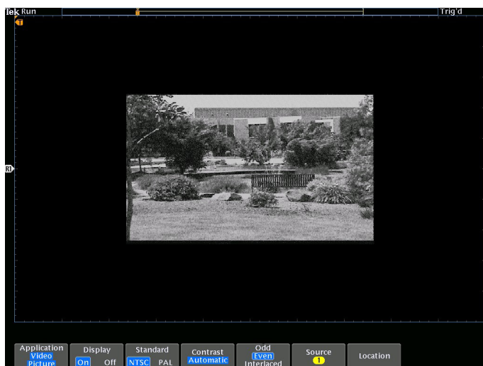
Viewing an NTSC video signal. Video picture mode contains automatic contrast and brightness settings as well as manual controls.
