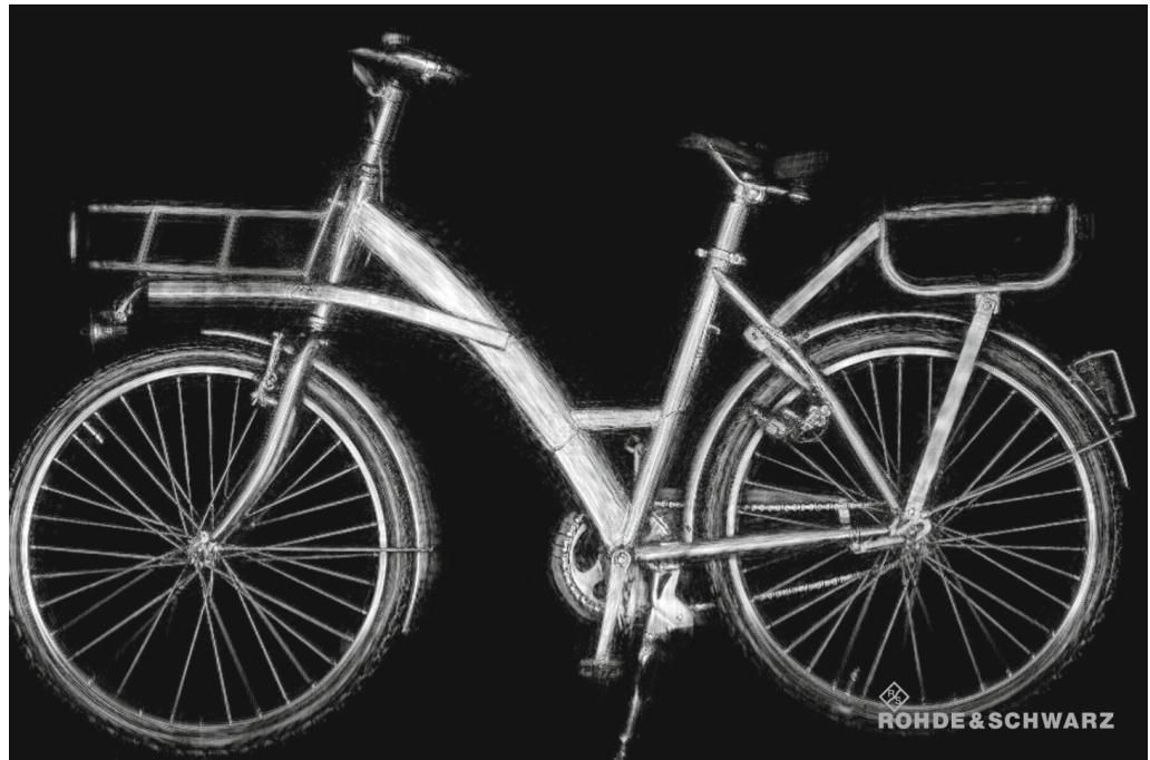
Fig. 10: mmWave picture taken by Rohde & Schwarz, frequency 70 GHz to 80 GHz, several thousand transmitting and receiving antennas
