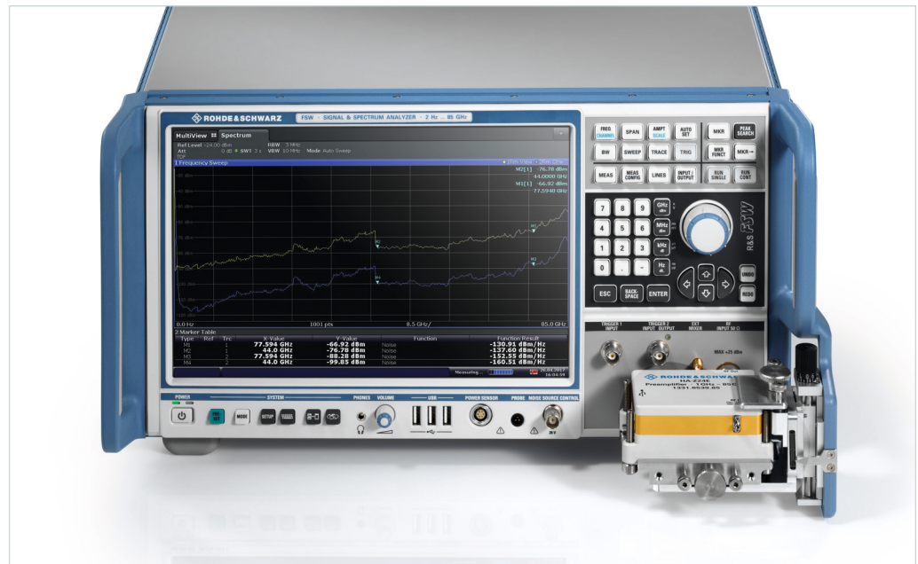
Fig. 5: R&S®FSW85 signal and spectrum analyzer with the R&S®HA-Z24E external preamplifier (1 GHz to 85 GHz)
