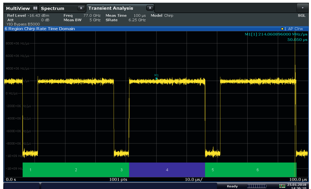
Fig. 12: Chirp rate measurement in the time domain used as a base for chirp detection
