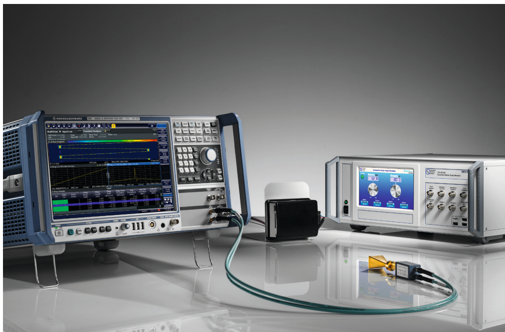
Fig. 2: The R&S®FSW26 (up to 26.5 GHz) can be used with the R&S®FS-Z90 external harmonic mixers (60 GHz to 90 GHz) to measure RF signals in the E band.
