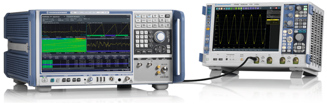
Fig. 6: The R&S®FSW85 signal and spectrum analyzer equipped with the R&S®FSW-B5000 hardware option used together with an R&S®RTO2064 oscilloscope as an external digitizer provides an equalized 5 GHz signal analysis bandwidth.
