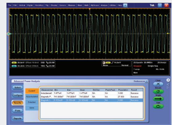
Magnetic Losses on an MSO5000B
